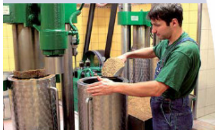
EXTRACTION OF OIL from sunflower kernels poses no special problem; therefore, an oil press can be employed successfully to squeeze the oil from the seed.
